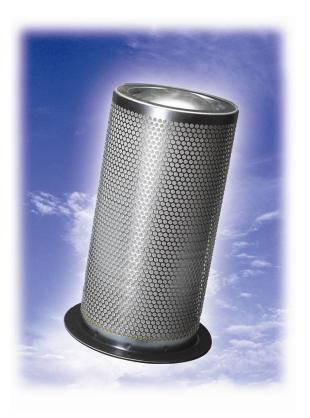
The standard conventional oil separator is the original design for the removal of oil aerosols from the compressed air stream. This element design consists of a specific amount of a uniform grade of borosilicate glass fibers, "wrapped" onto a support tube. When properly sized to the cfm/m3/min flowrate and corresponding operating pressure of the machine, this element will provide consistent performance according to the following data:
